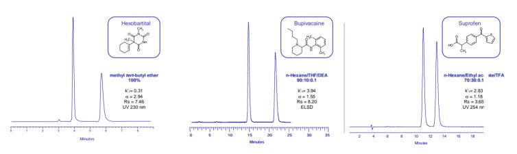
General conditions: CHIRALPAK® IA 250 x 4.6 mm, Flow rate: 1 ml/min, 25°C
